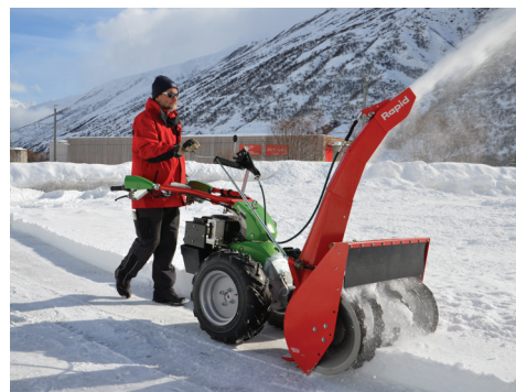
Target location for snow throwing can be conveniently adjusted via the handlebar during travel
