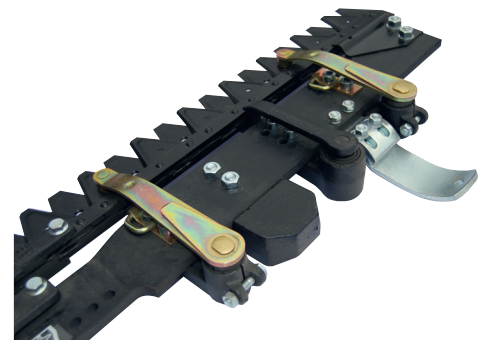
Dual cutter bars are equipped with additional weights and slip heels as standard
