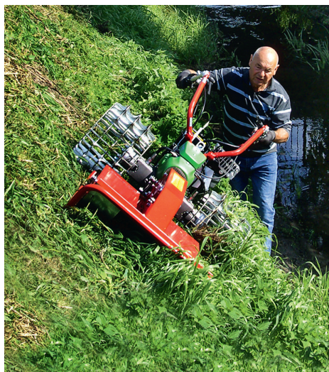
Robust, 8 mm thick steel blades
