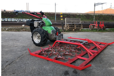
Towed attachment Due to the conceptual structure of the pasture harrow, it is possible to work comfortably trailing/pulling in the forward direction.
