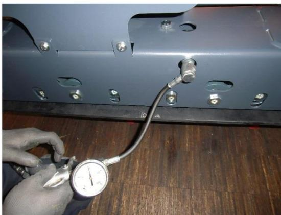
To check the track, place the sleeve coupling ③ of the grease gun on the flat grease nipple. The specified pressure should be 180 bar.
