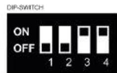
Compressor shuts down when 8 bar is reached, or maximum after 30 s.
