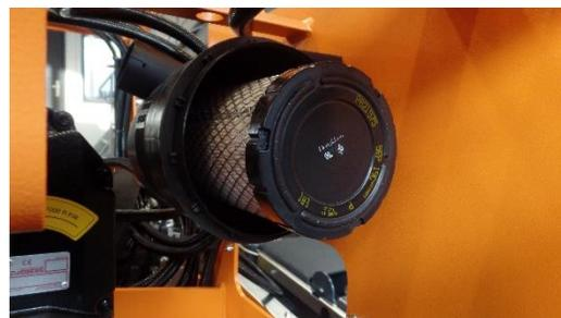
also pull out the safety cartridge by a slight twist and replace it each time, when the main cartridge is replaced.
