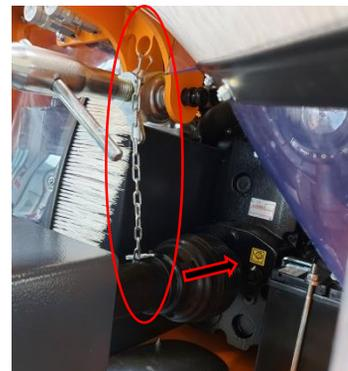
Secure the clamp lock & the drive shaft safety track to the frame and hook the drive shaft to the gearbox
