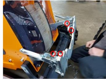
Fix **KAT.1 holder** via 4 bolts and nuts
