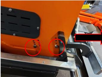
Loosen **original holder** by opening the side screw connection on the frame.
