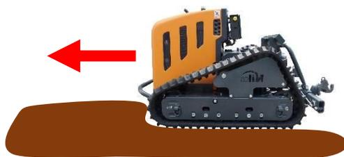
Do not move along the edge of a slope or uneven surface while one rubber track is in horizontal position and the other is tilted or partially raised. →If the machine is at an angle of more than 10°! Always drive the machine so that both tracks move on the same horizontal surface to avoid the risk of track damage.
