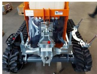
Hook in the Rapid holder & fold up the locking lever
