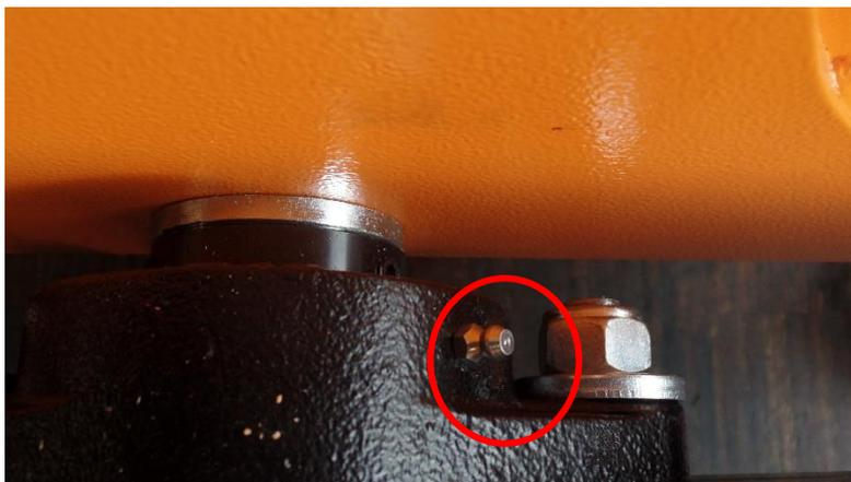
Lateral displacement lubrication only when the chassis is extended. Interval: **Annually**
