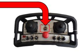
When starting the engine, the potentiometer setting should be set to 100%.
