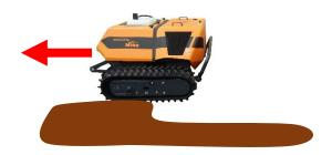
Do not move along the edge of a slope or uneven surface while one rubber track is in horizontal position and the other is tilted or partially raised.
