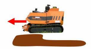
Do not move along the edge of a slope or uneven surface while one rubber track is in horizontal position and the other is tilted or partially raised.
