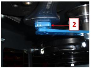
To tension the arm, a 30 mm openended spanner is required.
