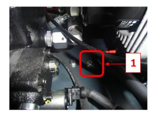
After slightly loosening the screw (1), return the tension arm (2) by turning it left to the default setting between 15° and 30°. Then tighten the screw (1).
