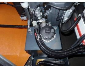
Always check the condition of all hydraulic lines and O-rings for leaks. For this purpose, a cardboard box can be placed underneath to detect any leaks. If leaks occur, replace the component to be replaced if it is defective or damaged.
