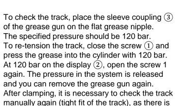
To relax, the grease nipple must be loosened until the necessary relaxation of the track becomes apparent.
